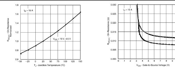
COMPARISON OF MODEL WITH MEASURED DATA (T, = 25 °C UNLESS OTHERWISE NOTED)
